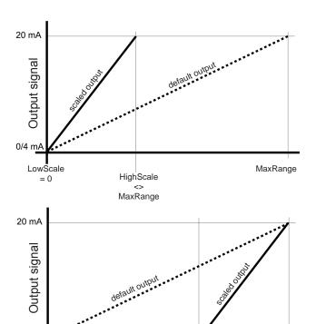
The "LowScale" and "HighScale" parameters allow a concentration value to be set to correspond to the lower (0 or 4 mA) or upper signal value (20 mA). The limis for these parameters are given by the "MinRange" and "MaxRange" parameters, specifying the physical measuring ranges of each instrument (\*\*\* 5.7.4.1, page 5-27).
